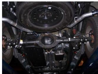
8. Install exit pipes #E onto tailpipes. Cut to your preferred length then use clamps to secure exit pipes to tailpipes.
