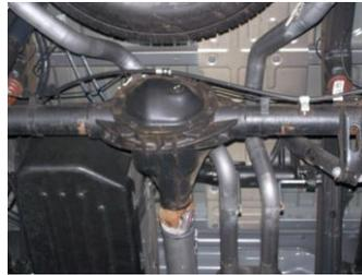
7. Install passenger side tailpipe #C into muffler at least 1.5" to 2". Use clamp #G to secure pipe to muffler. Do not tighten. The tailpipes will both lean towards the driver side for clearance. Insert welded hangers into rubber grommets.
