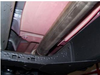
3. **2009 Models Only** Measure 8" from the flange on your new headpipe #A and cut. Attach adapter pipe to new headpipe with the 3" clamp. You will re-use the factory band clamp
