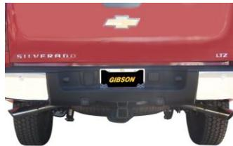
Install stainless steel tips. Clamp down. When you have everything in place, firmly tighten all bolts and clamps down securely. Use stainless steel cleaner and a Scotch Brite pad weekly to prevent tip from discoloration. Inspect all fasteners after 25-50 miles of operation and re-tighten as necessary.
