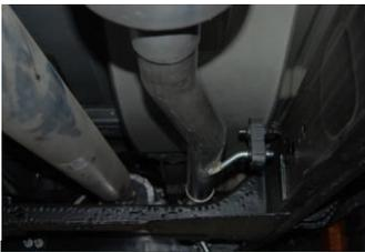
3. Bolt adapter #I to the stock flange re-using the factory into rubber grommet. Do not tighten.
