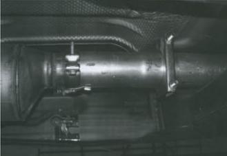
Next, install headpipe #A into adapter #I. Insert welded hanger into the rubber grommet. Use clamp #F to secure, do not tighten
