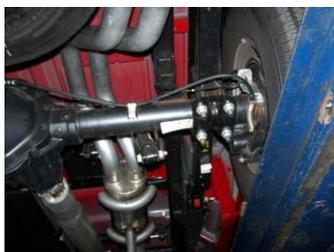
5. Slide the passenger side over axle tailpipe #C into the muffler 1.5-2". Use clamp #G to secure. Do not tighten. Insert welded hanger into rubber grommet.
