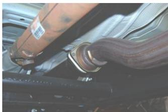
2. To remove your stock exhaust, unbolt the 2-bolt flange located in front of the muffler. Disengage the welded hangers from the rubber grommets. Use WD-40 to aid in this process. Do not remove or damage the rubber grommets as you will reuse them to mount your new system. Now, cut off tailpipe and remove exhaust. Do not throw away stock hardware.
