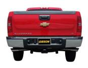
9. Install stainless steel tip. Clamp down. When you have everything in place, firmly tighten all bolts and clamps down securely. Use stainless steel cleaner and a Scotch Brite pad weekly to prevent tip from discoloration. Inspect all fasteners after 25-50 miles of operation and re-tighten.
