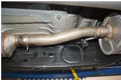
unbolt it at the clamp behind the Y-pipe. Make sure to leave all rubber grommets in the factory location. **You will re-use stock nuts and bolts.** For easier removal of exhaust, cut behind the muffler. Use WD-40 to remove hangers from grommets.
