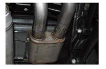
Lay out the exhaust on the floor so it looks like the drawing and compare parts with manual. To remove the stock exhaust remove it from the factory clamp in front of your stock muffler. Leave all rubber grommets in place. Use WD-40 to aid in removal of exhaust and hangers. Use hacksaw to cut tailpipe off for easier removal.
