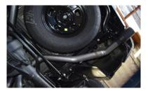
Install exit pipes # E Use clamps # H to secure exit pipes to tailpipes. The system is a universal kit and will require some adjusting to find the optimum position for your vehicle.
