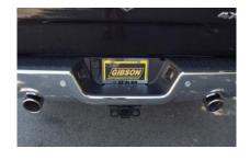
Now go back and tighten all clamps, nuts and bolts. Use stainless steel cleaner weekly to prevent tip from discoloration. Inspect all fasteners after 25-50 miles of operation and re-tighten as necessary.
