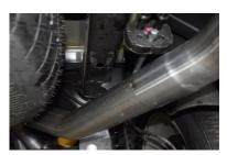
Install the passenger side tailpipe # C into the muffler at least 1-1/2" to 2". Use clamp # H to secure pipe to muffler. Do not tighten. The tailpipes both will lean towards the driver side for clearance.
