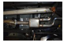
Install muffler onto head pipe # A 1-1/2" to 2". Use a jack stand to support the muffler. Use clamp #H to the secure the muffler to the head pipe. Do not tighten
