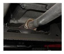
TO REMOVE THE STOCK EXHAUST UNBOLT IT FROM THE 2-BOLT FLANGE JUST BEHIND THE CONVERTER. FOR EASIER REMOVAL OF THE STOCK EXHAUST CUT THE STOCK TAILPIPE OFF JUST BEHIND THE MUFFLER. LEAVE ALL RUBBER **GROMMETS ON THE** HANGER. USE WD-40 TO AID IN REMOVAL OF THE EXHAUST AND HANGERS. **DO NOT DISGUARD** HARDWARE, YOU WILL **RE-USE IT.**
