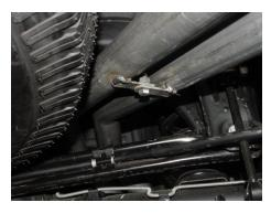
INSTALL DRIVERS SIDE TAILPIPE #C INTO THE MUFFLER 1-1/2" TO 2". USE BOLT KIT #H TO SECURE THE TAILPIPES TOGETHER. DO NOT TIGHTEN.
