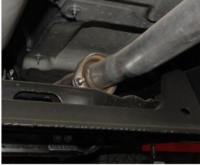
TO REMOVE THE STOCK EXHAUST UNBOLT IT FROM THE 2-BOLT FLANGE JUST BEHIND THE CONVERTER. FOR EASIER REMOVAL OF THE STOCK EXHAUST CUT THE STOCK TAILPIPE OFF JUST BEHIND THE MUFFLER. LEAVE ALL RUBBER GROMMETS ON THE HANGER. USE WD-40 TO AID IN REMOVAL OF THE EXHAUST AND HANGERS. **DO NOT DISGUARD HARDWARE, YOU WILL RE-USE IT.**
