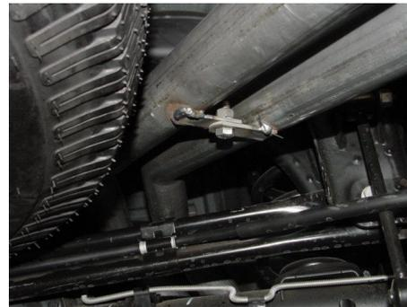
INSTALL DRIVERS SIDE TAILPIPE #C INTO THE MUFFLER 1-1/2" TO 2". USE BOLT KIT #H TO SECURE THE TAILPIPES TOGETHER. DO NOT TIGHTEN.
