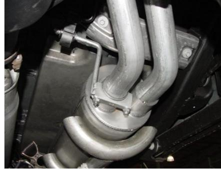
INSTALL PASSENGER SIDE TAILPIPE #D INTO MUFFLER 1-1/2 TO 2". INSERT WELDED HANGER INTO RUBBER GROMMET. USE CLAMP #I TO SECURE THE TAILPIPE TO THE MUFFLER. DO NOT TIGHTEN.
