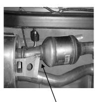
CUT BRACKET AT THIS POINT. THEN CUT 3/4" IN FRONT ON THE MUFFLER ON PASS. SIDE
