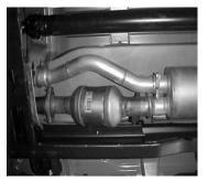
INSTALL HEADPIPE #A ON THE FACTORY DRIVERSIDE AND ATTACH HEADPIPE USING CLAMP #F. DO NOT TIGHTEN. INSTALL THE MUFFLER WITH THE OUTLET'S POSITIONED AT 12 O'CLOCK. INLET HAS LOUVERS FACING FORWARD TO CATCH THE EXHAUST. USE A JACKSTAND TO SUPPORT THE MUFFLER.
