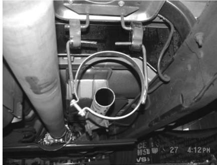
INSTALL THE BAND CLAMP #G INTO FACTORY GROMMETS BEHIND THE STOCK HEADPIPE. ATTACH WITH BOLT KIT #I. NEXT, SLIDE MUFFLER THROUGH THE BAND CLAMP WITH THE INLET TOWARDS THE MOTOR. USE CLAMP #E TO SECURE MUFFLER TO THE STOCK PIPE. USE A JACK STAND TO SUPPORT THE MUFFLER. INLET HAS LOUVERS INSIDE FACING TOWARDS THE MOTOR. DO NOT TIGHTEN
