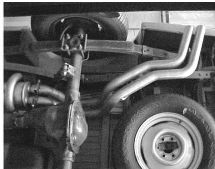
INSTALL DRIVERSIDE OVERAXLE TAILPIPE #C INTO MUFFLER AT LEAST 1  $\frac{1}{2}$ " TO 2". INSERT WELDED HANGER INTO RUBBER GROMMET. USE HANGER #F TO ATTACH TAILPIPE TO MUFFLER OUTLET. USE BOLT KIT #H TO BOLT BOTH TAILPIPES TOGETHER. DRIVERSIDE TAILPIPE BRACKET SHOULD BE ON TOP OF PASSENGER TAILPIPE BRACKET. DO NOT TIGHTEN.
