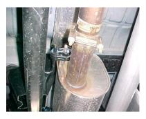
YOU MAY NEED TO HEAT IT UP FOR EASIER REMOVAL. LEAVE ALL RUBBER GROMMETS IN PLACE. USE WD-40 FOR REMOVAL OF HANGERS.
