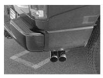
INSTALL YOUR BLACK CERAMIC COATED TIPS. PROCEED TO THE NEXT SHEET ON HOW TO INSTALL YOUR DEEGAN 38 BADGES. AFTER YOU HAVE CHECKED FOR CLEARANCES GO BACK AND TIGHTEN ALL NUTS, BOLTS AND CLAMPS.
