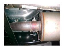
YOU MAY NEED TO HEAT IT UP FOR EASIER REMOVAL. LEAVE ALL RUBBER GROMMETS IN PLACE. USE WD-40 FOR REMOVAL OF HANGERS.
