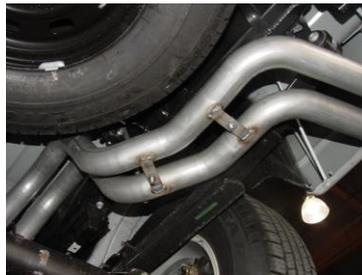
INSTALL PASSENGER SIDE TAILPIPE #D INTO MUFFLER AND ATTACH USING CLAMP #F. INSERT WELDED HANGER INTO RUBBER GROMMET. DO NOT TIGHTEN. USE BOLT KIT #I TO ATTACH THE TAILPIPES TOGETHER. DO NOT TIGHTEN. PASSANGER SIDE TAB ON THE TAILPIPE WILL BE ON TOP OF THE DRIVERSIDE TAB.
