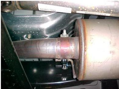
**DO NOT REMOVE YOUR HEADPIPE.** YOU MAY NEED TO HEAT IT UP FOR EASIER REMOVAL. LEAVE ALL RUBBER GROMMETS IN PLACE. USE WD-40 FOR REMOVAL OF HANGERS.
