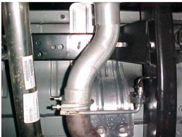
INSTALL HEADPIPE #A ONTO YOUR EXISTING STOCK FRONT PIPE AND SECURE WITH CLAMP #K. INSERT WELDED HANGER INTO RUBBER GROMMET.
