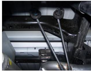
**3.** Insert welded hangers into rubber grommets.
