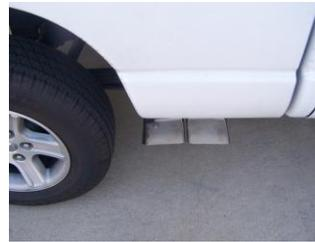
**4.** Install stainless steel tips. Clamp down. When you have everything in place, firmly tighten all bolts and clamps down securely. Use stainless steel cleaner and a Scotch Brite pad weekly to prevent tip from discoloration. Inspect all fasteners after 25-50 miles of operation and re-tighten as necessary
