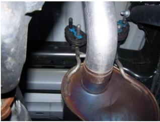
**1.** To remove the stock exhaust remove it from in front of the stock muffler. Disengage the welded hangers using WD-40 from the OEM rubber grommets. Do not damage or remove the rubber grommets as you will re-use them to mount your new system. Now, cut off tailpipe and remove exhaust.
