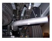
**5.** Install the passenger side overaxle tailpipe #C into the muffler 1½"-2". Use clamp #H to secure tailpipe to muffler. DO NOT TIGHTEN. Insert welded hanger into rubber grommet.
