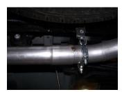
**7.** Install the driver overaxle tailpipe #D into the muffler 1½-2". Use clamp #H to secure. Use another clamp #H to hold pipe up to hanger. DO NOT TIGHTEN.
