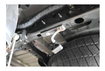
**5.** Then, install Hanger Bracket **#J** using supplied Bolt Kit **#I** on DS of frame. (Use sample photo for reference)
