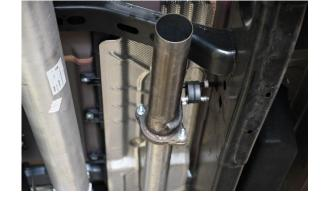
**1.** To remover the factory exhaust you will need to loosen the clamp located above the rear axle.
