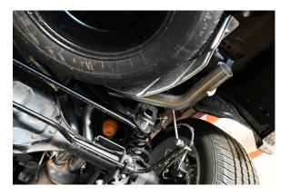
**4.** Now, install PS Overaxle Pipe **#C** and DS Overaxle Pipe A **#D** with supplied clamps **#K** (KEEP CLAMPS A BIT LOOSE AS THIS KIT HAS FLEXIBILITY WITH FITMENT).
