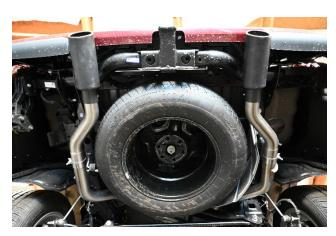
7. Finally, install Exit Pipes **#F** with supplied clamps **#K** and Tips **#G**. Once Tips are in desired location you may begin to start tightening from front to back.
