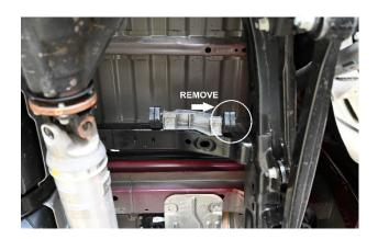
**3.** Next, remove passenger side rubber grommet used to mount muffler and install it on hanger bracket **#J.** Then install muffler assy. **#B** with supplied clamp **#L.**
