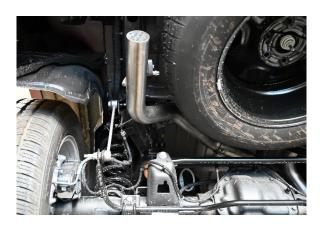
**6.** Once Hanger Bracket is secured you may install DS Overaxle Pipe B **#E** with supplied clamp **#K**. **(CLAMPS ARE TO REMAIN A BIT LOOSE TO AID IN FINAL FITMENT)**
