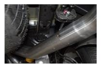
Install the passenger side tailpipe # C into the muffler at least 1-1/2" to 2". Use clamp #J to secure pipe to muffler. Do not tighten.
