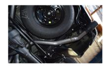
Install exit pipes # E and #F Use clamps #I to secure exit pipes to tailpipes. The system is a universal kit and will require some adjusting to find the optimum position for your vehicle. Sometimes the muffler outlets may need to be rotated slightly to help find the perfect fit.
