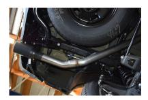
Install the Gibson Tips onto your exit pipes. Place the tips to your desired position. Be for tightening down the system it is recommended to secure the tips in the position you want and check the location after each connection is tightened.
