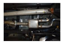
Install muffler onto head pipe # A 1-1/2" to 2". Use a jack stand to support the muffler. Use clamp #I to the secure the muffler to the head pipe. Do not tighten
