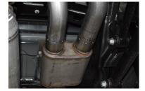
Install head pipe # A Use a jack stand to support the factory exhaust. Do not tighten.
