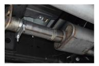
Lay out the exhaust on the floor so it looks like the drawing and compare parts with manual. To remove the stock exhaust remove it from the factory flange in front of your stock muffler. Leave all rubber grommets in place. Use WD-40 to aid in removal of exhaust and hangers. Use hacksaw to cut tailpipe off for easier removal.
