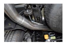
Install the driver side tailpipe # D into the muffler at least 1-1/2" to 2". This pipe will route over the axle and between the Frame rail and tire. Use clamp #J to secure pipe to the muffler. Do not tighten.
