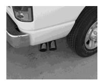
Install band clamp #H onto muffler with hanger rods facing forward and insert hangers into rubber grommet. **Do not tighten.**
