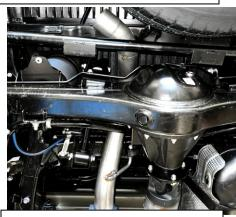
5. Install your over axle pipe and insert the hanger in to grommet and remove muffler support. Do not tighten
