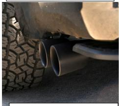
7. Be sure to check all clearance after each section has been tightened to be sure there is proper clearance. It may take 4-500 miles for your vehicle to fully adjust to the changes in exhaust flow.
