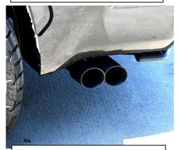
6.Install your exit pipe and exhaust tips. Now go back and adjust the kit so you have proper clearance and the muffler sits level with the frame rail, the tips were designed to have the tips 1" below the ½ panel. Begin to tighten from the front to the back. Check clearance as parts will
