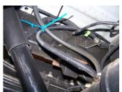
9. Zip tie brake lines and fuel hoses away from pipes. (see picture)
