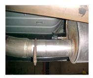
2. Remove your stock exhaust by removing the clamp located in front of your stock muffler. Disengage the welded hangers from the OEM rubber grommets. Use WD-40 to aid in this process. Do not damage or remove the rubber grommets as you will reuse them to mount your new system. Now, cut off tailpipe and remove exhaust.
