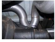
5. Install the passenger side tailpipe #C to the muffler assembly 1.5-2". Use clamp #F to secure. Insert welded hanger into rubber grommet.
