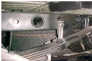
ON DRIVER SIDE: ATTACH REAR TAILPIPE HANGER #I TO FRAME BY REMOVING THE 18MM HITCH BOLT. THEN RE INSTALL BOLT WITH HANGE (IF YOU DO NOT HAVE A FACTORYHITCH USE BOLT KIT #L TO ATTACH HANGER #I TO THE FRAME RAIL. REPEAT ON PASSENGER SIDE.
