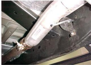
INSTALL HEADPIPE # A INTO STOCK PIPE. THE END OF THE PIPE SHOULD BE AT THE 12 O'CLOCK POSITION, ATTACH WITH FACTORY CLAMP. DO NOT TIGHTEN. INSERT WELDED HANER INTO RUBBER GROMMET.
