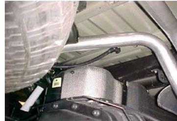
INSTALL DRIVERS SIDE TAILPIPE # D INTO MUFFLER 1 1/2" TO 2". INSERT WELDED HANGERS INTO RUBBER GROMMETS. USE CLAMP # H TO SECURE PIPE TO MUFFLER, DO NOT TIGHTEN.
