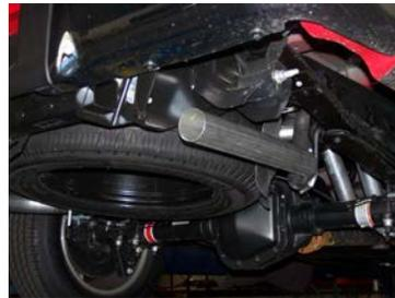
INSTALL EXIT PIPES # E ONTO TAILPIPES. ROTATE OUT TO THE SIDES; ATTACH TO TAILPIPES WITH CLAMPS # H.
