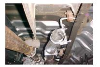
INSTALL HEADPIPE # A ONTO FACTORY PIPE. LINE UP THE NOTCH. USE CLAMP # H TO SECURE HEADPIPE TO FACTORY PIPE. DO NOT TIGHTEN. NEXT INSTALL FRONT MUFFLER HANGER #F ONTO HEADPIPE. SLIDE WELDED HANGER INTO RUBBER GROMMET. USE THIS CLAMP TO SECURE MUFFLER TO HEADPIPE. DO NOT TIGHTEN.
