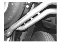
NEXT INSTALL PASSENGER OVER AXLE PIPE # C INTO MUFFLER 1½ TO 2" IT WILL ROUTE UNDERNEATH PASSENGER SIDE TAILPIPE, AND ATTACH TO MUFFLER WITH CLAMP # G. USE BOLT KIT # I TO SECURE PIPES TOGETHER. WELDED TABS ON PASSENGER TAILPIPE WILL BE ON TOP OF OTHER PIPE TABS.
