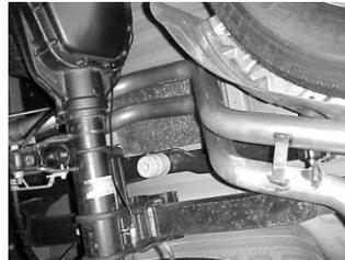
**NEXT INSTALL DRIVERS OVER AXLE PIPE # D INTO MUFFLER 1 1/2" TO 2". USE CLAMP # F TO SECURE PIPE TO MUFFLER. DO NOT TIGHTEN. USE BOLT KIT # I TO SECURE PIPES TOGETHER. DRIVERSIDE TAB WILL BE ON THE BOTTOM.**
