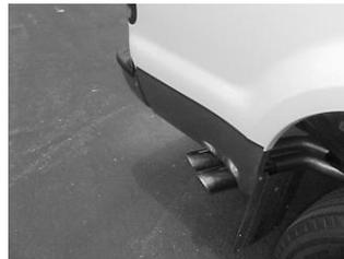
**INSTALL YOUR STAINLESS TIPS. TIGHTEN ALL CLAMPS STARTING FROM THE FRONT, WORKING YOUR WAY TO THE BACK OF THE TRUCK. TO CLEAN TIPS USE A STAINLESS STEEL CLEANER & SCOTCH BIE PAD.**
