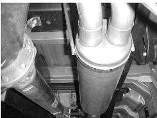
**SLIP MUFFLER # B THROUGH BAND CLAMP THEN ONTO THE HEADPIPE 1 1/2" TO 2". THE OUTLETS WILL BE LEVEL. USE CLAMP # G TO SECURE MUFFLER TO HEADPIPE. DO NOT TIGHTEN.**
