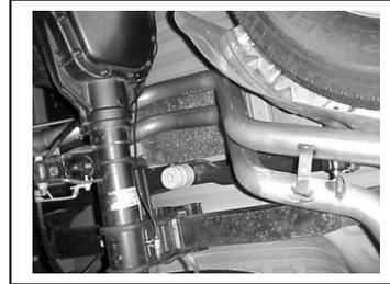
NEXT INSTALL DRIVERS OVER AXLE PIPE # D INTO MUFFLER 1 1/2 TO 2". USE CLAMP # F TO SECURE PIPE TO MUFFLER. DO NOT TIGHTEN. USE BOLT KIT # H TO SECURE PIPES TOGETHER. DRIVERSIDE TAB WILL BE ON THE BOTTOM.
