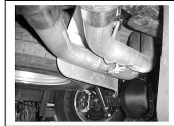
INSTALL DRIVER SIDE OVER AXLE TAILPIPE # D INTO MUFFLER 1 1/2 TO 2". INSERT WELDED HANGER INTO RUBBER GROMMET, USE CLAMP # G TO SECURE PIPE TO MUFFLER. THIS PIPE WILL GO INTO THE DRIVERS SIDE OUTLET. DO NOT TIGHTEN
