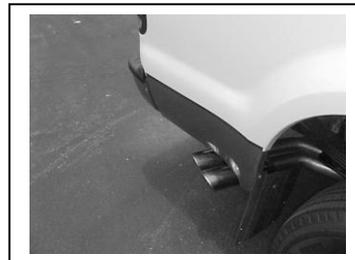
INSTALL YOUR BLACK CERAMIC COATED TIPS. PROCEED TO THE NEXT SHEET ON HOW TO INSTALL YOUR DEEGAN 38 BADGES. AFTER YOU HAVE CHECKED FOR CLEARANCES GO BACK AND TIGHTEN ALL NUTS,
