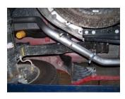
**4.** Install the passenger side overaxle tailpipe #C into the muffler 1½"-2". Use clamp #H to secure tailpipe to muffler. DO NOT TIGHTEN. Insert hanger into rubber grommet.
