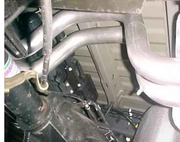
INSTALL PASS. SIDE TAILPIPE # C INTO MUFFLER 1 1/2" TO 2". INSERT HANGER INTO RUBBER GROMMET, USE CLAMP # G TO SECURE PIPE TO MUFFLER. DO NOT TIGHTEN. YOU MAY NEED TO LOOSEN AND PUSH OVER TOWARDS THE DRIVERS SIDE AND RE-TIGHTEN.
