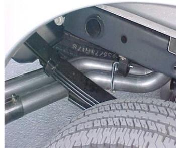
INSTALL DRIVERS SIDE TAILPIPE # D INTO MUFFLER 1 1/2" TO 2". INSERT HANGER INTO RUBBER GROMMET, USE CLAMP # G TO SECURE PIPE TO MUFFLER. DO NOT TIGHTEN. THE TAB ON THIS PIPE SHOULD GO ON TOP OF PASSENGER SIDE PIPE USE BOLT KIT # J TO SECURE TOGETHER.
