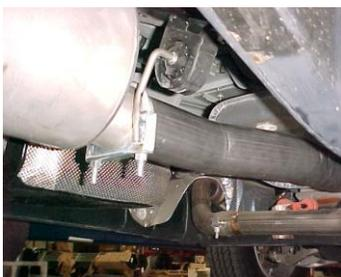
INSTALL FRONT MUFFLER HANGER # F ONTO MUFFLER INLET, INSERT HANGER INTO RUBBER GROMMET, DO NOT TIGHTEN. USE BOLT KIT # I TO SECURE.
