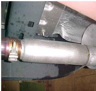
INSTALL HEADPIPE # A INTO STOCK PIPE. THE END OF THE PIPE SHOULD BE AT THE 9 O'CLOCK POSITION, USE CLAMP # H TO SECURE PIPES TOGETHER, DO NOT TIGHTEN.
