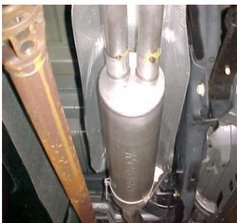
INSTALL MUFFLER # B ONTO HEADPIPE 1 1/2" TO 2". USE A JACK STAND TO HOLD UP THE MUFFLER. OUTLETS SHOULD BE ON THE TOP.
