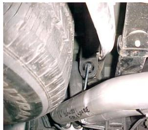
INSTALL PASS. SIDE TAILPIPE # C INTO MUFFLER 1 1/2" TO 2". INSERT HANGER INTO RUBBER GROMMET, USE CLAMP # G TO SECURE PIPE TO MUFFLER. DO NOT TIGHTEN.
