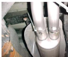
INSTALL DRIVERS SIDE TAILPIPE # D INTO MUFFLER 1 1/2" TO 2". INSERT HANGERS INTO RUBBER GROMMETS, USE CLAMP # G TO SECURE PIPE TO MUFFLER. DO NOT TIGHTEN. THE TAB ON THIS PIPE SHOULD GO ON BOTTOM OF PASSENGER SIDE PIPE USE BOLT KIT # H TO SECURE TOGETHER.
