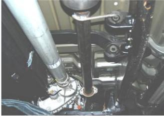
INSTALL HEADPIPE # A INTO STOCK PIPE. THE END OF THE PIPE SHOULD BE AT THE 12 O'CLOCK POSITION, ATTACH WITH BOLT KIT #I DO NOT TIGHTEN. INSERT WELDED HANGER INTO RUBBER GROMMET. REMOVE THE HANGER FROM THE FRAME & RELOCATE TO THE HOLES JUST TO THE LEFT OF THE OTHER HOLES YOU WILL NEED TO PRY THE INSERTS OUT & RE-INSTALL SEE PHOTO
