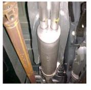
INSTALL MUFFLER # B ONTO HEADPIPE 1 ½" TO 2". USE CLAMP # G TO SECURE MUFFLER TO HEADPIPE. DO NOT TIGHTEN. USE A JACK STAND TO HOLD UP THE MUFFLER. OUTLETS SHOULD BE LEVEL.
