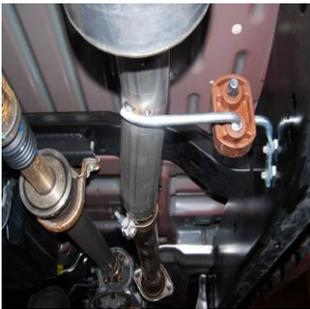
INSTALL HEADPIPE #A ONTO STOCK FLANGE. INSERT WELDED HANGER INTO RUBBER GROMMET. USE BOLT KIT PROVIDED TO SECURE. DO NOT TIGHTEN.
