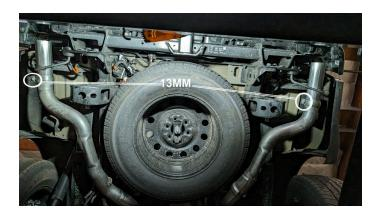
1) FIRST, REMOVE BOTH DRIVER AND PASSENGER SIDE FACTORY TIPS. THEY ARE HELD ON BY A 13MM BOLT.
