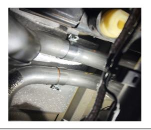
2) SECOND, LOOSEN BOTH 15MM CLAMPS LOCATED ABOVE THE AXLE THEN REMOVE BOTH OVER-AXLE PIPES.
