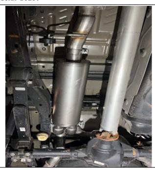
3) THIRD, LOOSEN THE 15MM CLAMP ATTACHING THE MUFFLER TO THE HEADPIPE, THEN REMOVE THE MUFFLER ASSEMBLEY. ONCE REMOVED, INSTALL HEADPIPE #A ALONG WITH MUFFLER #B USING CLAMP #G. (SNUG DOWN CLAMP, DON'T TIGHTEN)
