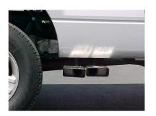
INSTALL STAINLESS TIPS, THEN TIGHTEN ALL NUTS, BOLTS, AND CLAMPS.
