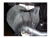
NEXT, REMOVE THE TWO BOLTS THAT HOLD THE HEAT SHIELD ON, THEN INSTALL THE REAR HANGER # E , RE-USING THE FACTORY BOLTS. ATTACH USING CLAMP # D.
