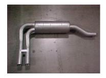
NEXT, INSTALL MUFFLER ASSEMBLY # A INTO STOCK HEADPIPE AND ATTACH WITH CLAMP # D.
