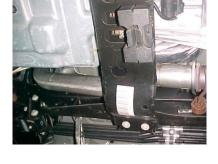
INSTALL PIPE # N ONTO PIPE # O. USE CLAMPS #K TO SECURE PIPES TOGETHER. DO NOT TIGHTEN.
