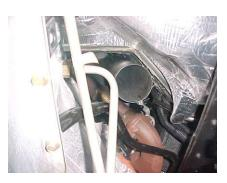
INSTALL PIPE #J O ONTO TURBO RE- USING YOUR STOCK CLAMP. DO NOT TIGHTEN.
