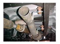
2. INSTALL HEADPIPE #A ONTO STOCK HEADPIPE, LINE UP THE NOTCH AND INSERT WELDED HANGERS INTO RUBBER GROMMETS USE CLAMP # K TO SECURE PIPES TOGETHER. DO NOT TIGHTEN. LEAVE LOOSE FOR EASIER INSTALLATION.
