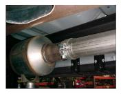
1. To remove the stock exhaust disengage the welded hangers using WD-40 from the OEM rubber grommets. Do not damage or remove the rubber grommets as you will re-use them to mount your new system. Now, cut off tailpipe and remove exhaust.
