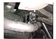
**5.** Install passenger side over axle tailpipe #D into the muffler 1½-2" and secure with clamp #H. Insert welded hanger into rubber grommet. DO NOT TIGHTEN.
