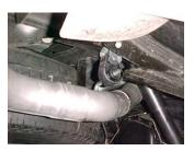
**5.** Install passenger side over axle tailpipe #D into the muffler  $1\frac{1}{2}-2^{"}$  and secure with clamp #H. Insert welded hanger into rubber grommet. DO NOT TIGHTEN.
