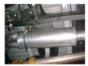
**3.** Install band clamp #G into rubber grommets located above the axle and attach bolt kit #M. DO NOT TIGHTEN. Install muffler #B onto headpipe 1½-2" with the louvers facing the converter. Secure with clamp #L. DO NOT TIGHTEN. Use a jack stand to support the muffler.
