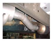
**2.** Install headpipe #A onto your catalytic converter and attach with clamp #K. Use a jack stand to support the converter. DO NOT TIGHTEN. Insert welded hanger into rubber grommet.
