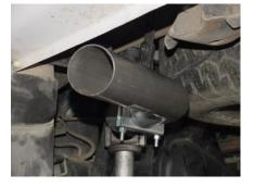
INSTALL DRIVERS SIDE TAILPIPE #B INTO MUFFLER 1-1/2" TO 2". ROTATE TAILPIPE UNTIL IT TOUCHES HANGER #J. ATTACH HANGER # H TO TAILPIPE. INSTALL EXIT PIPE #C AND ATTACH TO HANGER #J AND TO THE TAILPIPE WITH CLAMP #I. DO NOT TIGHTEN.
