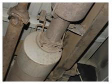
TO REMOVE THE STOCK EXHAUST UN-CLAMP IT JUST IN FRONT OF THE MUFFLER. YOU MAY NEED TO HEAT IT UP TO REMOVE IT. NOW CUT OFF YOUR STOCK TAILPIPE JUST AFTER THE MUFFLER. FOR EASIER REMOVAL FO STOCK HANGERS USE WD-40. LEAVE ALL RUBBER GROMMETS IN PLACE.
