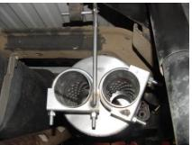
INSTALL MUFFLER #A ONTO STOCK PIPE WITH THE NOTCH ON THE TOP. INSTALL FRONT MUFFLER HANGER #G. INSERT HANGERS INTO RUBBER GROMMETS. USE THIS CLAMP TO SECURE MUFFLER TO STOCK HEADPIPE. DO NOT TIGHTEN.
