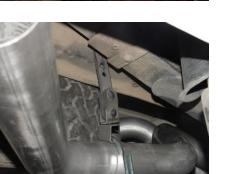
INSTALL HANGER #J ONTO FRAME BY MEASURING 23" FROM THE REAR OF THE FRAME. ON BOTH SIDES YOU WILL FIND A 3/8" HOLE. USE THIS HOLE TO BOLT ON YOUR NEW HANGER. INSTALL BOLT KIT #J ON THE 3<sup>RD</sup> HOLE FROM THE BOTTOM.
