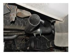
INSTALL PASSENGER SIDE TAILPIPE #D INTO MUFFLER 1-1/2" TO 2". USE CLAMP #I TO SECURE PIPE TO MUFFLER. DO NOT TIGHTEN. ROTATE TAILPIPE UNTIL IT TOUCHES HANGER #J. INSTALL EXIT PIPE #E AND ATTACH TO HANGER #J AND TO THE TAILPIPE WITH CLAMP #I. DO NOT TIGHTEN.
