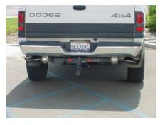
INSTALL THE STAINLESS TIPS. TO CLEAN TIPS USE ANY STAINLESS OR ALUMINUM CLEANER AND A SCOTCH BRITE PAD. NOW GO BACK AND TIGHTEN ALL CLAMPS STARTING FROM THE FRONT AND WORKING BACK.
