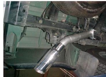
INSTALL EXIT PIPES # E ONTO TAILPIPES USE CLAMP # I TO SECURE PIPES TOGETHER. DO NOT TIGHTEN. ON DRIVER SIDE USE CLAMP #I TO SECURE PIPE TO REAR HANGER #J.
