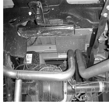
INSTALL THE DRIVERSIDE FRONT TAILPIPE # D TO OUTLET OF MUFFLER NOT MORE THAN 1.5" TO 2". THE TAILPIPE INLET THAT GOES INTO THE MUFFLER IS 4.5" LONG. ATTACH WITH HANGER# G. INSTALL DRIVERSIDE OVERAXLE TAILPIPE # E TO FRONT DRIVERSIDE TAILPIPE, THIS PART HAS A SWEDGE UP ON IT. ATTACH USING CLAMP # G. INSTALL PASSENGER OVERAXLE TAILPIPE TO THE OUTLET OF THE MUFFLER NOT MORE THAN 1.5" TO 2". THE TAILPIPE INLET THAT GOES INTO THE MUFFLER IS 4.5" LONG AND ATTACH WITH CLAMP # G. DO NOT TIGHTEN.
