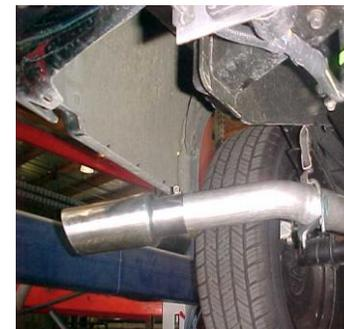
CUT 5 INCHES OFF EACH EXIT PIPE, THEN INTSTALL EXIT PIPES # F TO THE OVERAXLE TAILPIPES, USE CLAMP #G TO SECURE. USE ZIP TIES FOR BRAKE AND HOSE LINES TO KEEP AWAY FROM PIPES. NOW FIRMLY TIGHTEN ALL BOLTS, CLAMPS AND HANGERS. INSTALL YOUR STAINLESS TIPS TO YOUR DESIRED LOOK.
