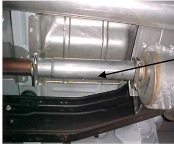
INSTALL NEW HEADPIPE #A AND ATTACH USING CLAMP #G TO FACTORY PIPE.
