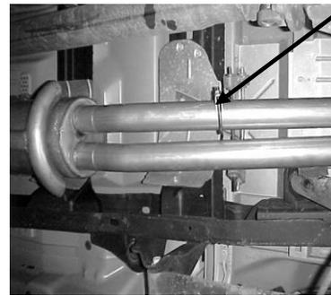
NEXT INSTALL HANGER # J TO DRIVERSIDE TAILPIPE AND INSERT WELDED HANGER INTO RUBBER GROMMET.MAKE SURE YOU HAVE EQUAL SPACE BETWEEN SHOCK AND SPARE TIRE. THE SPARE TIRE MAY NEED TO BE LOOSEND AND PUSH TO THE DRIVER SIDE AND THEN ROTATE THE OVERAXLE PIPE TO GAIN CLEARANCE.
