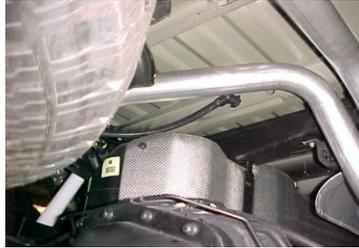
INSTALL DRIVERS SIDE TAILPIPE # D INTO MUFFLER 1 1/2" TO 2". INSERT WELDED HANGERS INTO RUBBER GROMMETS. USE CLAMP # H TO SECURE PIPE TO MUFFLER, DO NOT TIGHTEN.
