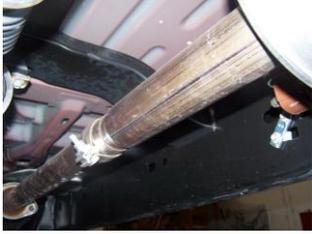
TO REMOVE YOUR STOCK EXHAUST, REMOVE IT FROM FLANGE LOCATED JUST IN FRONT OF THE MUFFLER REMOVE HANGERS FROM RUBBER GROMMETS BY PULLING EXHAUST TOWARDS THE REAR OF THE VEHICLE, USE WD-40 TO AID IN REMOVAL, LEAVE GROMMETS IN PLACE.
