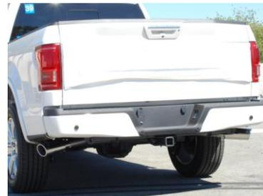
INSTALL YOUR STAINLESS TIPS AND CUT YOUR EXIT PIPES TO YOUR DESIRED LOOK AND LENGTH\*\* THEN GO BACK AND TIGHTEN ALL CLAMPS, ROTATE SYSTEM FOR BEST CLEARANCE BEFORE TIGHTENING.
