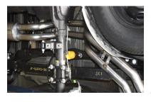
INSTALL PASSENGER SIDE OVER AXLE TAILPIPE # C INTO MUFFLER 1½ TO 2". INSERT WELDED HANGER INTO RUBBER GROMMET, USE CLAMP # G TO SECURE PIPE TO MUFFLER. THIS PIPE WILL GO INTO THE PASSENGER SIDE OUTLET. DO NOT TIGHTEN
