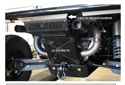
4. Then, remove factory bumper by unbolting the 2 bolts in the center of the bumper. Once removed, reinstall the bumper with **Beauty Plate B** between the frame and bumper mount plate re-using factory hardware. Leave bolts loose while you install **Bolt Kit D** onto the beauty plate. Once all bolts are in, center the plate and tighten all hardware. (**WE RECOMMEND USING A M6 X 1.0 TAP ON THE REAR 4 HOLES USED TO MOUNT THE BEAUTY PLATE TO CLEAN THE THREADS.**)
