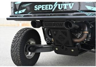
5. Lastly, install both Tips C to desired outlet length and tighten down. (You may need to loosed bumper bolts and adjust bumper to get equal tip spacing.)
