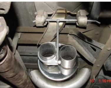
INSTALL MUFFLER #B ONTO HEADPIPE 1-1/2" TO 2". OUTLET SHOULD BE LEVEL. USE CLAMP #J TO SECURE MUFFLER TO HEADPIPE. DO NOT TIGHTEN. INSTALL REAR MUFFLER HANGER #G ONTO THE DRIVERSIDE MUFFLER OUTLET. INSERT HANGERS INTO RUBBER GROMMETS. DO NOT TIGHTEN.
