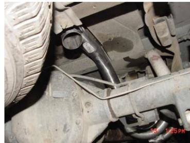
INSTALL DRIVERSIDE FRONT TAILPIPE #D INTO MUFFLER 1-1/2" TO 2". SECURE TO MUFFLER WITH HANGER #G. INSTALL TAILPIPE #E ONTO FRONT PIPE, USE CLAMP #I TO SECURE TOGETHER. DO NOT TIGHTEN.
