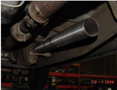
INSTALL HEADPIPE #A ONTO FACTORY PIPE USING CLAMP #K TO SECURE TOGETHER. DO NOT TIGHTEN.
