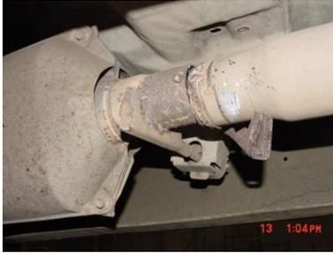
**TO REMOVE STOCK EXHAUST UNBOLT THE CLAMP LOCATED JUST BEHIND THE CATALYTIC CONVERTER.** FOR EASIER REMOVAL CUT THE STOCK TAILPIPE OFF JUST BEHIND THE MUFFLER AND REMOVE. LEAVE ALL RUBBER GROMMETS ON THE HANGER. USE WD-40 TO AID IN REMOVAL OF EXHAUST AND HANGERS.
