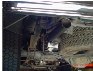
INSTALL EXIT PIPES #F ONTO TAILPIPES, ROTATE THE PIPE UNTIL IT IS AT THE PROPER LOOK FOR YOU. USE CLAMPS #I TO SECURE PIPES TOGETHER. DO NOT TIGHTEN.
