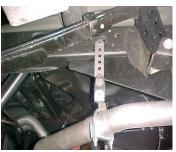
ON DRIVER SIDE MEASURE 17-1/2" FROM THE REAR OF THE FRAME FORWARD. USE HANGER # I. USE THE TOP HOLE OF THIS HANGER. USE HARDWARE PROVIDED.
