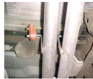
INSTALL THE DRIVERSIDE FRONT TAILPIPE # D TO OUTLET OF MUFFLER 1.5" TO 2". THE TAILPIPE INLET THAT GOES INTO THE MUFFLER IS 4.5" LONG. INSERT HANGER INTO RUBBER GROMMET. INSTALL DRIVERSIDE OVERAXLE TAILPIPE # E TO FRONT DRIVERSIDE TAILPIPE, THIS PART HAS A SWEDGE UP ON IT. ATTACH USING CLAMP # G.
