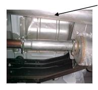
INSTALL NEW HEADPIPE #A AND ATTACH USING CLAMP #G TO FACTORY PIPE.
