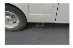
8. INSTALL YOUR STAINLESS TIPS. THEN GO AND TIGHTEN ALL OF THE NUTS, BOLTS, AND CLAMPS FROM TE FRONT WORKING YOUR WAY BACK.
