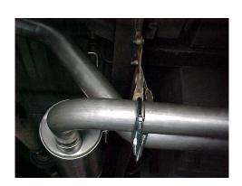
6. INSTALL PASSENGER SIDE TAILPIPE #E INTO MUFFLER 1 1/2" – 2", AND USE CLAMP #H TO HOLD TAILPIPE TO 10" HANGER. DO NOT TIGHTEN.
