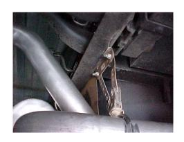
5. INSTALL BOTH 10" HANGERS #J, ONTO BRACKET WHERE YOUR STOCK ONE WAS MOUNTED. YOU WILL USE THE TOP HOLE, AND LEAVE IT LOOSE UNTIL TAILPIPES ARE INSTALLED.
