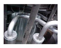
7. INSTALL DRIVERS SIDE TAILPIPE #D INTO MUFFLER 1 ½" – 2" IT WILL ROUTE OVER YOUR DRIVE SHAFT AND COME OUT ON THE RIGHT SIDE OF THE PASSENGER SIDE TAILPIPE. USE CLAMP #H TO SECURE TAILPIPE TO MUFFLER. USE CLAMP #H TO HOLD TAILPIPE UP TO 10" HANGER. DO NOT TIGHTEN! BOLT TAILPIPE TABS TOGETHER, DRIVERSIDE TAB WILL BE ON THE BOTTOM.
