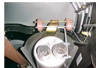
Install rear muffler T-hanger # I into rubber grommets located just above the muffler outlets. Shorter side of the hanger will be inserted on the passenger side grommet. Slide clamp onto passenger side muffler outlet. Do not tighten.
