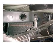
ON DRIVER SIDE: ATTACH REAR TAILPIPE HANGER #I TO FRAME BY REMOVING THE 18MM HITCH BOLT. THEN RE INSTALL BOLT WITH HANGER
