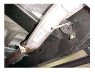
INSTALL HEADPIPE # A INTO STOCK PIPE. THE END OF THE PIPE SHOULD BE AT THE 12 O'CLOCK POSITION, ATTACH WITH FACTORY CLAMP. DO NOT TIGHTEN. INSERT WELDED HANGER INTO RUBBER GROMMFT.
