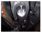
INSTALL MUFFLER # B ONTO HEADPIPE 1 ½" TO 2". USE CLAMP # G TO SECURE MUFFLER TO HEADPIPE, DO NOT TIGHTEN, USE A JACK STAND TO HOLD UP THE MUFFLER, OUTLETS SHOULD BE LEVEL.
