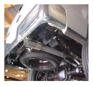
INSTALL EXIT PIPES # E ONTO TAILPIPES. ROTATE UNTIL LEVEL, USE CLAMP # H TO SECURE PIPES TOGETHER. DO NOT TIGHTEN.
