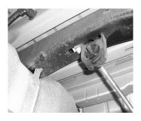
INSTALL WELDED HANGER INTO RUBBER GROMMET
